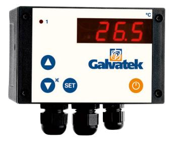
Number of setpoints: 1 Output contact: 1 changeover switch Supply voltage: 230V~. Max. switching voltage : 250V~ Max. breaking capacity : 12A Max. switching power : 2.6 kW
