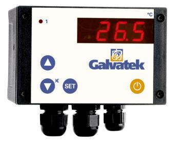
Number of setpoints: 1 Output contact: 1 changeover switch Supply voltage: 230V~. Max. switching voltage : 250V~ Max. breaking capacity : 12A Max. switching power : 2.76 kW / 230V
